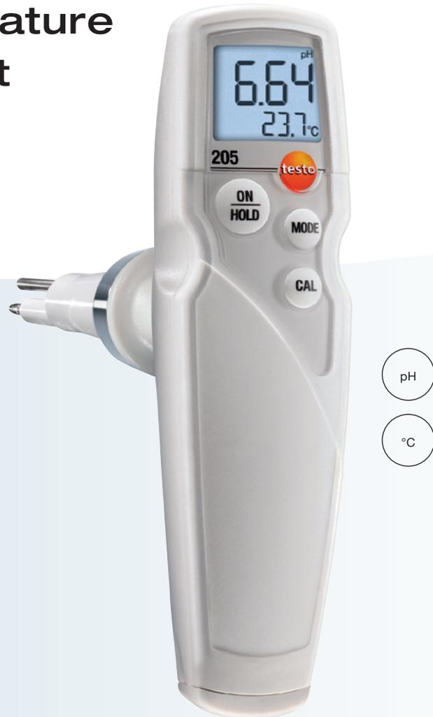
The testo 205 is a robust food penetration measuring instrument for temperature and pH values, with automatic temperature compensation. The robust penetration measurement tip is exchangeable and insensitive to dirt thanks to the hole diaphragm.
